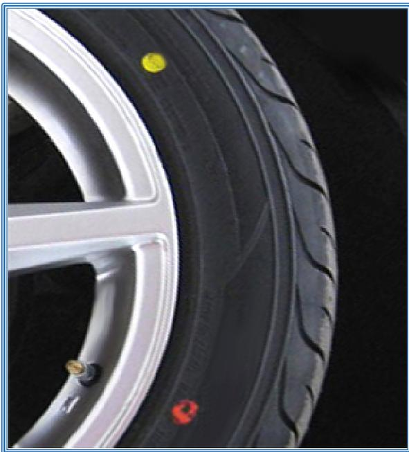
The **Yellow** dot indicates where the manufacturer has identified the lightest spot on the tire. This helps the balance technician match that spot to the heaviest spot on the rim—which is almost always where the valve stem is mounted. By aligning the valve stem and the **Yellow** dot, a wheel has a better chance of being more easily balanced.
